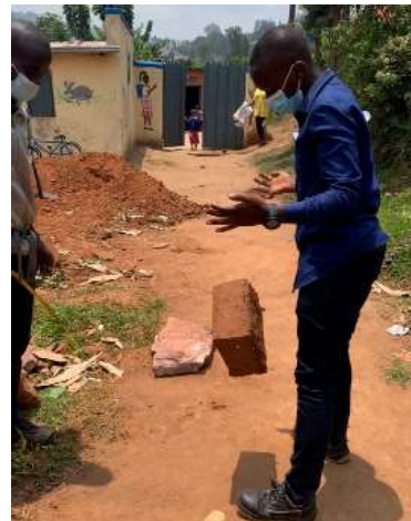
Figure 43(b). Dropping block on its corner
