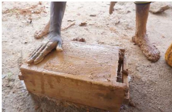
c) Smoothing top surface with water to finish
