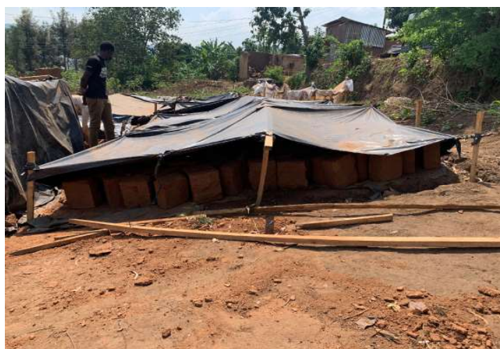
Figure 13. Block curing through air drying
