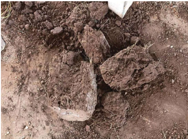
Shattered block: fail
