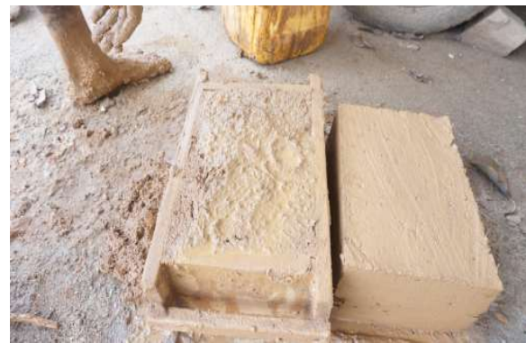
b) Once compacted, sprinkling the top with water
